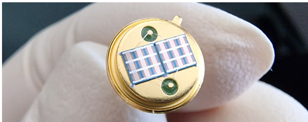
Infrared emitter array for thermal radiation between 2 and 15 \mu\text{m} up to 100 Hz.. Source: CiS
